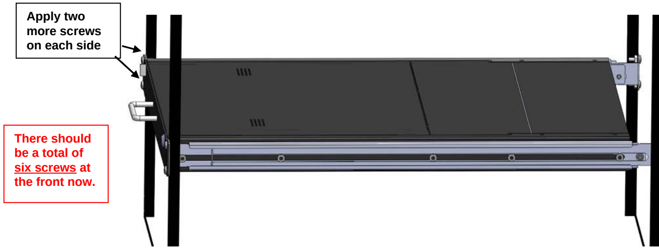
Figure 6- Apply remaining screws to complete installation
